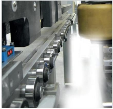
Laser photocell for reading origin and "tail" of the panel: The Skipper V31 compensates for any dimensional errors by correcting the X machining operation positions.
